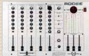
THE RODEC MX180 MKII introduced in 1997. The most important adjustments were the integration of RFI filters on all inputs needed to get CE approval.
